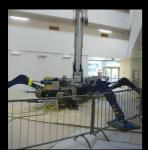
Variable jacking allowed the machine to set up in the small area of the atrium.
