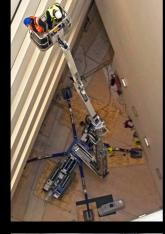
The FS420 Spider was able to fit through the narrow entrances to gain access to the atrium and was also able to reach the height required. Tracks allowed the machine to negotiate steps en route to the work area.
