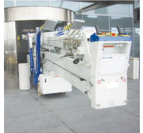
The FS 290, the narrowest in its class at 0.79m, fitted through the narrow doorway.
