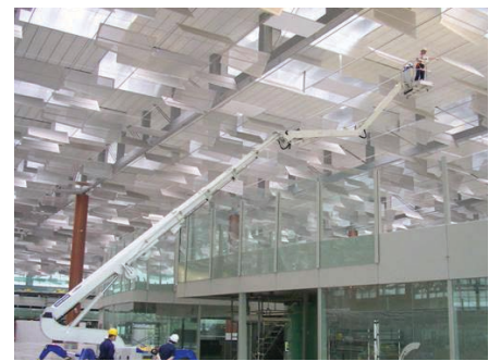
The FS 290, the narrowest in its class at 0.79m, fitted through the narrow doorway.
