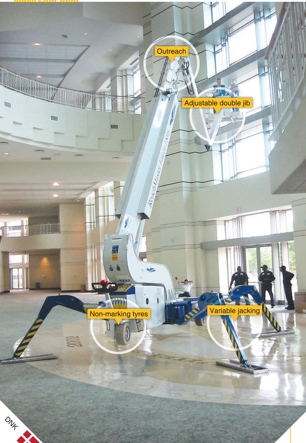
The FS 290, the narrowest in its class at 0.79m, fitted through the narrow doorway.
